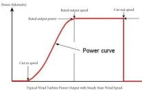
Wind turbines use either stall regulated or pitch regulated to avoid the fluctuations on the grid that results from high wind speed.
